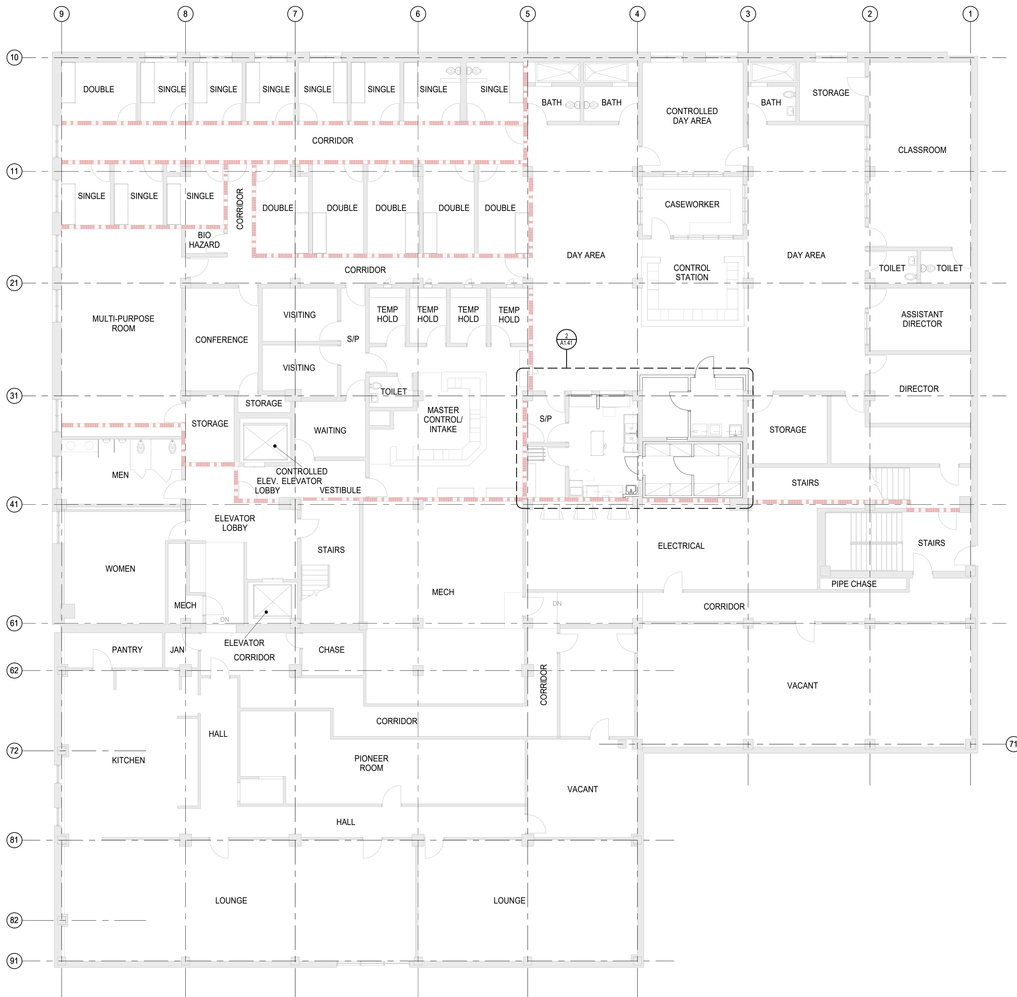
FOURTH FLOOR CODE ANALYSIS PLAN 1/8" = 1'-0"
